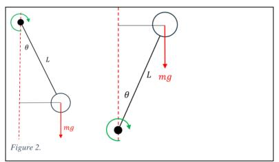
Let's take Galileo's pendulum on the left. The downward force on the bob due to gravity produces a torque around the pivot point
