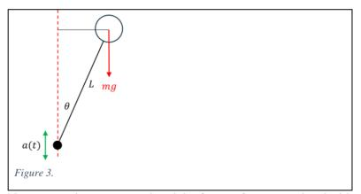
Now we can jump to a non-inertial reference frame associated with the oscillating axis, we can see that gravity g is supplemented by an additional acceleration due to the oscillating (and therefore accelerating pivot). We can then replace g in the equation of motion with
