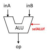
(a) Code up the ALU functionality, using the table of what the **op** will be according to the **sel\_ALUf** signal which directs the ALU what to do. You'll need a chain of **when** ... **else** ... **when**
