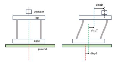
On the left is the equilibrium situation before the earthquake. The colored dotted lines indicate the starting location of the building components, all are aligned, there are no displacements. On the right is the situation during an earthquake; the building base is displaced relative to the ground; the top floor is displaced relative to the base and the damper is displaced relative to the top.
