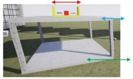
It's important to understand the output variables from the simulation. The computation generates a displacement of the building base, **dispB** relative to the ground. It then computes the displacement of the top floor **dispT** relative to the building base, and the displacement of the damper **dispD** relative to the top floor.
