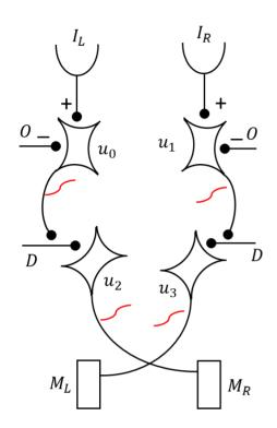
the bottom the left and right motors. You can also see the 'crossover' connexions which make this a vehicle type 2**b**.
