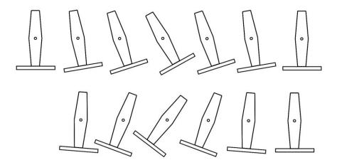
On the real ride, the operator has a joystick which he manipulates to add rotational force ('torque') to the centre of the arms from electric motors. In our model we shall use a periodic function (sine wave) since this removes the human out of the loop and makes investigations more controllable. Here's the idea.
