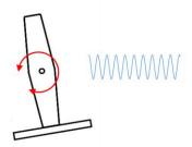
You can see the sine wave torque applied to the motor (blue curve) to force it first clockwise then anti-clockwise.
