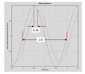
(b) Now re-run the script for the same desired phase lag and select corrected amplitude. You should get a phase-lagged sine wave with no amplitude change.
