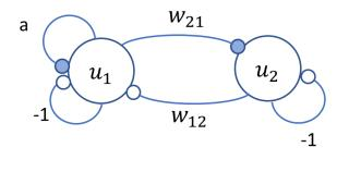
Remember empty synapses are inhibitory (negative) and filled synapses are excitatory. The inhibitory 'synapses' labelled -1 are modelling the leak in the bucket. Here the weight from neuron 1 to neuron 2,  $w_{21}$  is a positive number and the weight from 2 to 1 is negative, i.e.,  $w_{21} < 0$
