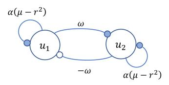
Here, the parameters  $\alpha$ ,  $\mu$ ,  $\omega$  are all fixed in time, and r is a variable given by  $r = \sqrt{u_1^2 + u_2^2}$ . The parameter  $\omega$  is the angular velocity of oscillation in rads/sec and ris the radius of the circle in the phase plane
