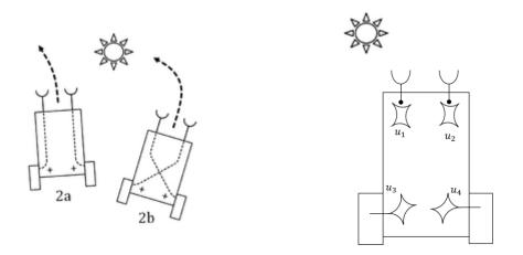
There are two sensory neurons  $u_1$  and  $u_2$  and two motor neurons  $u_3$  and  $u_4$ . Let's figure out how to build a neural circuit so the vehicle is attracted to the light (2b).
