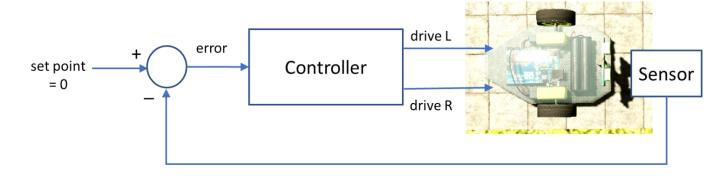
Let's see how the system works and therefore the code we must write. All symbols are explained at the end of this document. The maths model for the motors looks like this. The inputs to the motors from the controller are  $u_L$  and  $u_R$ , and each motor responds by providing a torque  $\tau_L$  and  $\tau_R$ . Details of these expressions will be provided later
