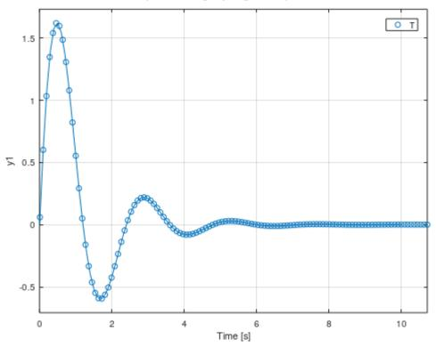
You see the controller responds by driving the angular velocity of the pole which then makes the angle theta approach zero.
