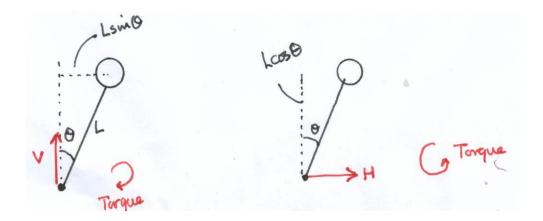
First the rotation about the centre of mass of the pendulum. The torque on the pendulum due to force *V* in the clockwise sense is calculated as force times the perpendicular distance to the centre of rotation.
