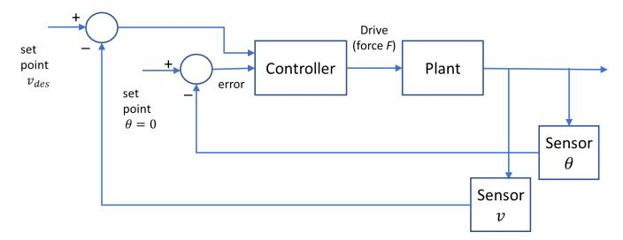
So we generate a second error signal for the controller from a velocity sensor attached to the Segway, and the set-point desired velocity.
