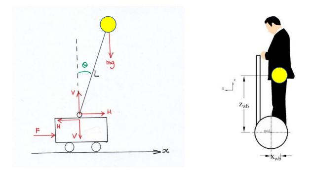
On the left is a picture of an inverted pendulum on a cart and on the right is a guy on a Segway. These two systems are identical where the yellow pendulum bob corresponds to the yellow centre of mass of the guy on the right.
