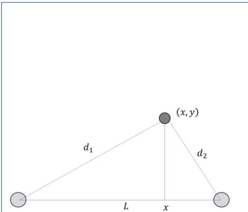
The origin is at the left beacon. The distance between the two beacons is  $L$ . The distances measured by the sensors (or computed from their readings) are  $d_1$  and  $d_2$ . Use Pythagoras theorem applied to the two triangles to find an expression for  $x$  in terms of  $d_1$ ,  $d_2$  and  $L$ . Ask for help if you like.
